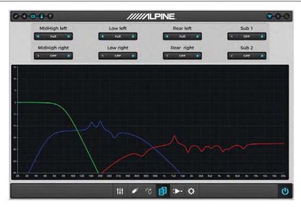
This screen visualizes the response curve(s) of the selected user adjustments of crossover, EQ, TCR and level for each output channel.
