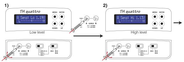
TURN THE KNOB TO REGULATE THE LEVEL OF THE A CHANNELS.
