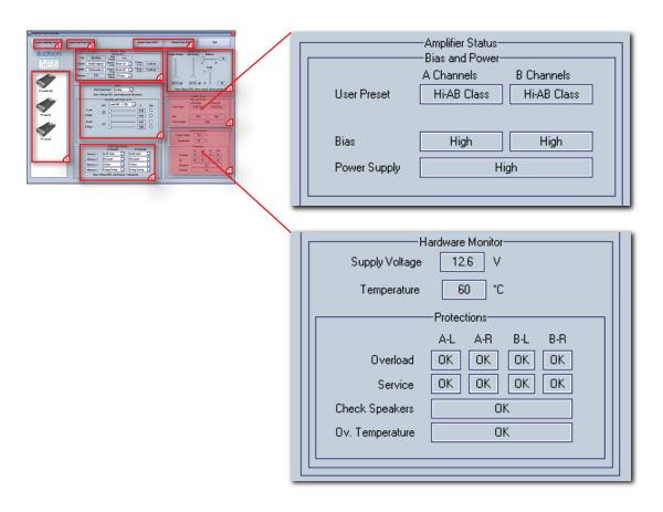
The ACNet software performs a real-time check-up of the amplifiers operating conditions.
