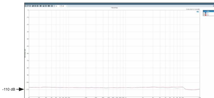
THD+N vs. frequency response @ 10 Watts / 4 Ohms
