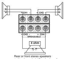
connected to channels 1 / 2 and subwoofer to channels 3 / 4.
