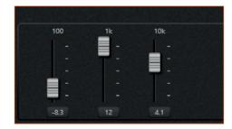
The central frequency of each band is indicated above the slider and the gain can be set with the slider or using text box below the slider.
