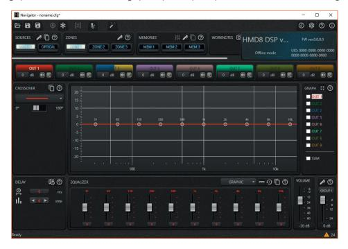
As you can see, the input channels panel and the zone volume panel are hidden, while the output channels panel takes on a reduced graphic layout.
