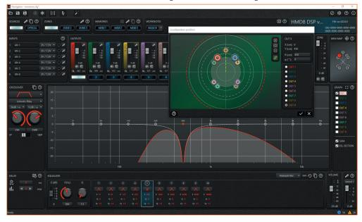
The software was designed to be adopted by all products with onboard DSP in the Hertz marine catalog and future ones: when you connect the device to the software, it automatically configures itself to display the interface of that specific device connected.
