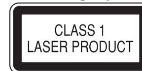
The label is attached to the chassis/case and says that the component uses laser beams that have been classified as Class 1. It means that the unit is utilizing laser beams that are of a weaker class. There is no danger of hazardous radiation outside the unit.
