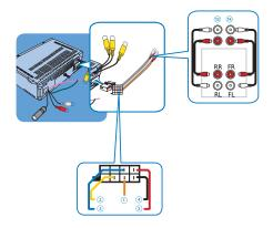
1 Illumination switch 2 To the +12V car battery which is energized at all time 3 Motor/electric antenna relay control lead/ Amplifier relay control lead 4 Ground 5 Ignition Key +12V DC when ON/ACC 6 Antenna 7 Aux-In 8 Parking Switch Cable 9 Reverse Driving Cable 10 Video-In
